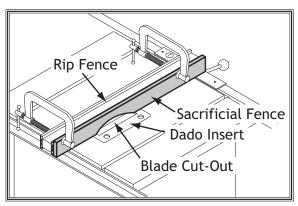
Figure 55. Sacrificial fence installed.
